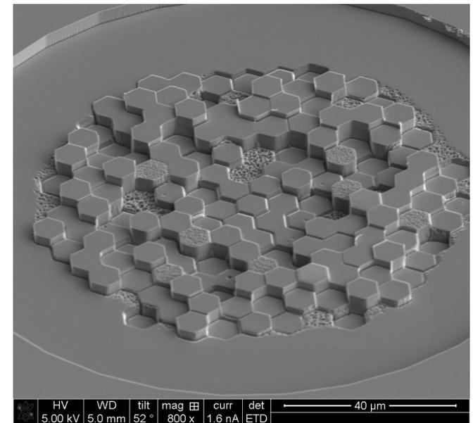
*Multi-zone focal plane mask. Each zone imprints an optical pathlength delay. Mutual interference between zones creates deep achromatic null. (credit: NAOJ/CNF)*
