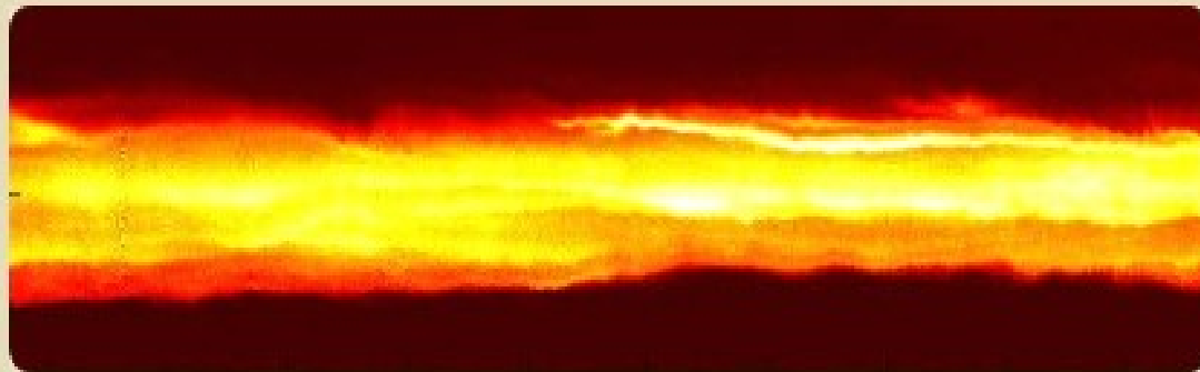
This image shows sodium density above the facility as a function of altitude (75 to 105 km) and time (horizontal direction, covering about 5 hours) on the night of August 5, 2008.
