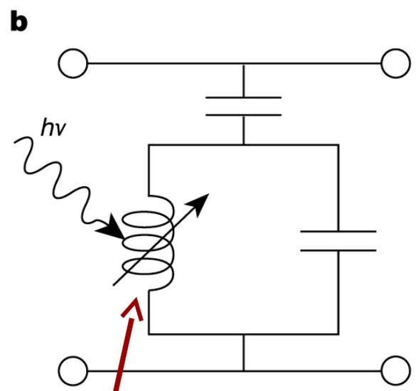
Inductor is a Superconductor!
