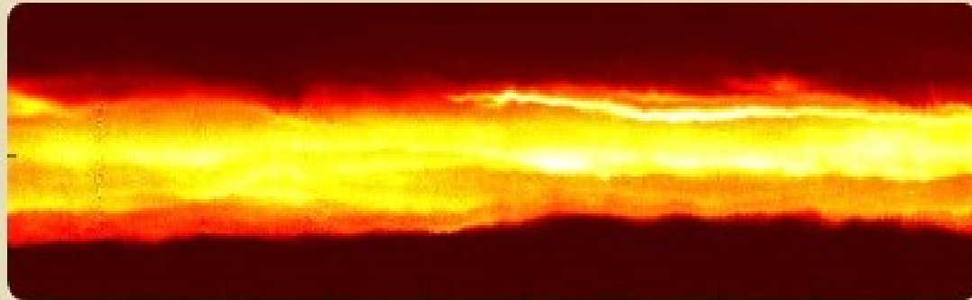
This image shows sodium density above the facility as a function of altitude (75 to 105 km) and time (horizontal direction, covering about 5 hours) on the night of August 5, 2008.
