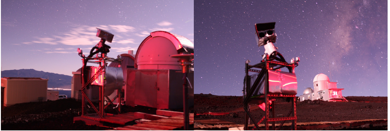
Figure 1. Left: Image of the robotic camera system on Mauna Loa observatory. Mauna Kea, to the North, can be seen in the background on the left. The cameras are mounted on an equatorial motorized mount on top of a metallic frame. The domes on the right host the VYSOS project robotic telescopes. Right: View pointing South. The Mauna Loa solar observatory is in the background. Openings for the two objectives can be seen on the front of the cameras enclosure. Note that the system does not have a dome, and simply points down during daytime or bad weather. The small shiny box on the right of the camera system is hosting humidity, temperature and cloud sensors.
