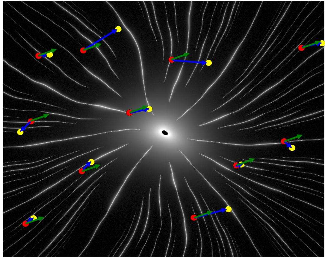
The measured astrometric motion (blue vectors in previous slide) is the sum of the true astrometric signal (green vectors) and the astrometric distortion induced by change in optics and detector between the 2 observations.
