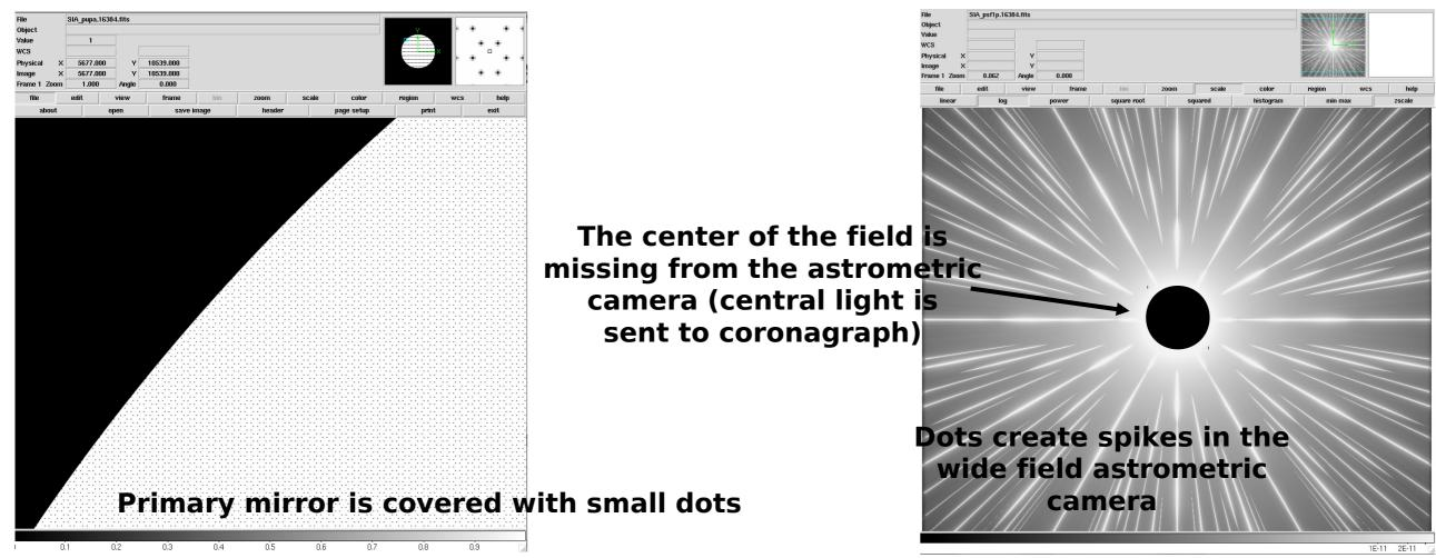
All astrometric distortions (due to change in optics shapes of M2, M3, and deformations of the focal plane array) **are common to the spikes and the background stars**. By referencing the background star positions to the spikes, the astrometric measurement is largely immune to large scale astrometric distortions.
