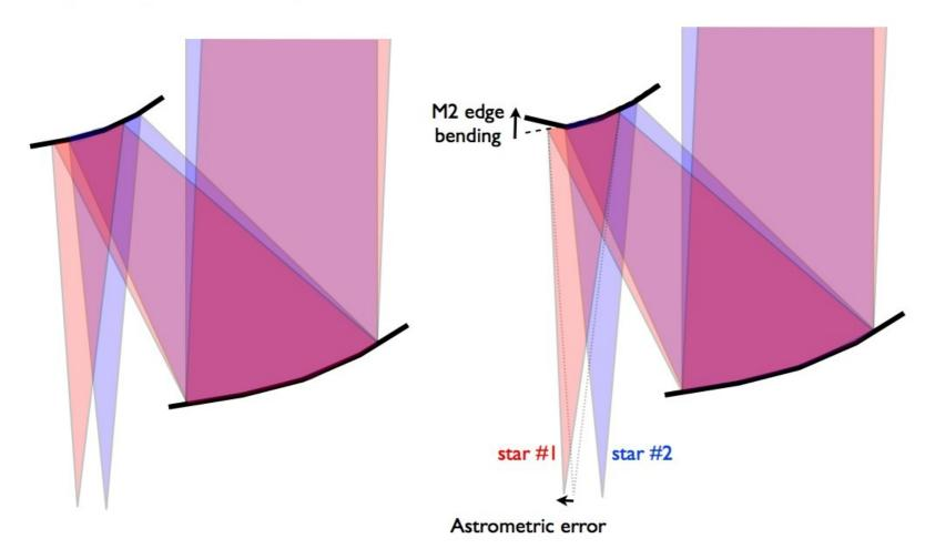
(1) Light from different stars on the sky travels different paths  $\rightarrow$ small bending of optics produces field distortions
