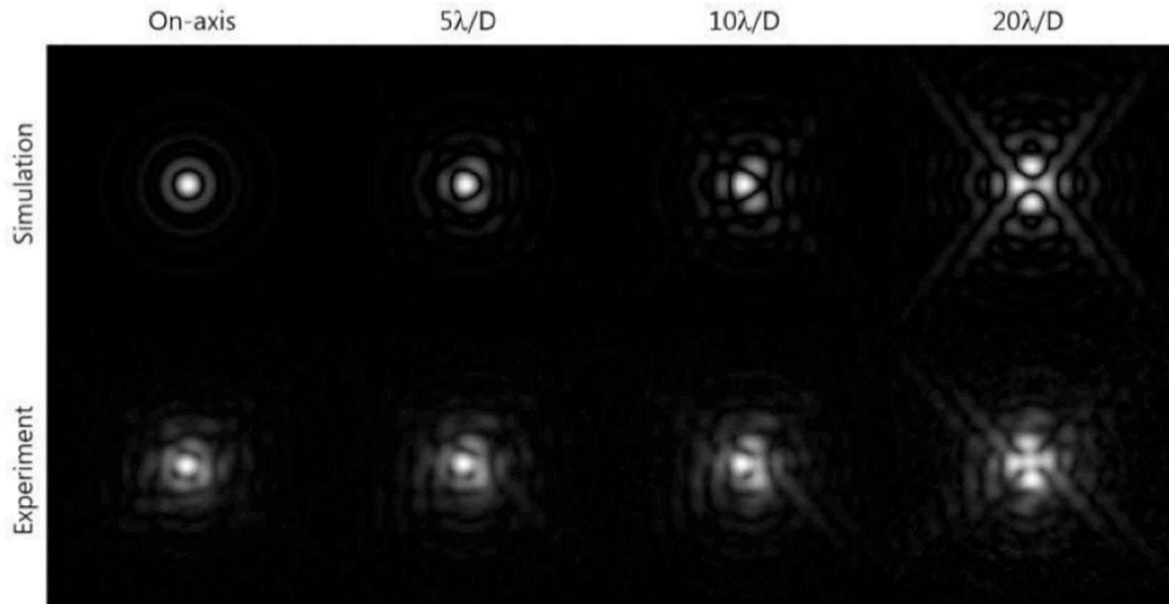
Fig. 12.— Comparison between simulated and experimental images of an off-axis source, from 0 to  $20 \lambda/D$  with a  $5 \lambda/D$  step. The field of view of each image is  $\pm 12\lambda/D$ .
