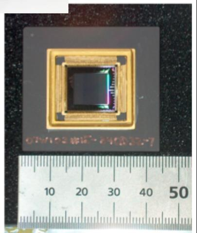
Figure 1: 1024 actuator (32x32) MEMs DM commercially available from Boston Micromachines (mm scale).
