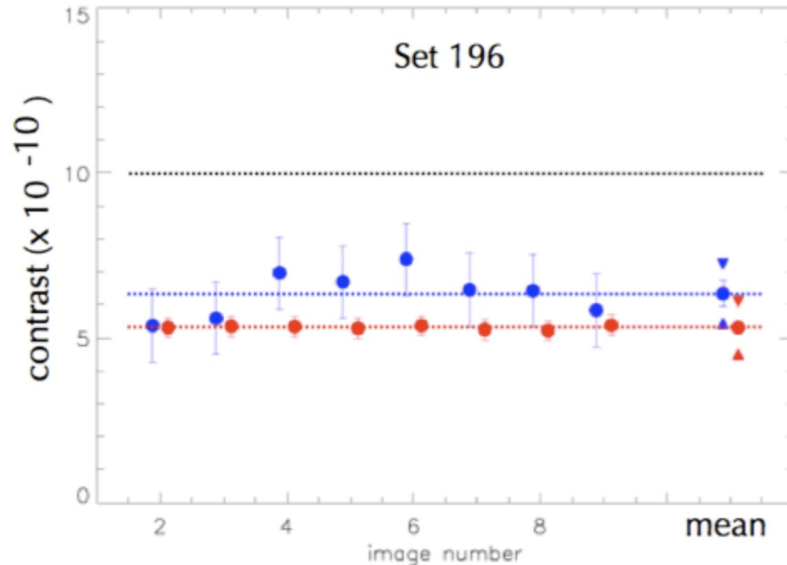
Contrast obtained in a sequence of images over a representative one-hour period. At left is the high contrast field: the inner and outer target areas are highlighted in blue and red respectively; an asterisk marks the location of the occulted “star”. Plotted at right are contrast values averaged over the inner and outer areas (again in blue and red respectively) for each image in the sequence.  $1-\sigma$  error bars indicate the measurement noise estimated from pairwise data.
