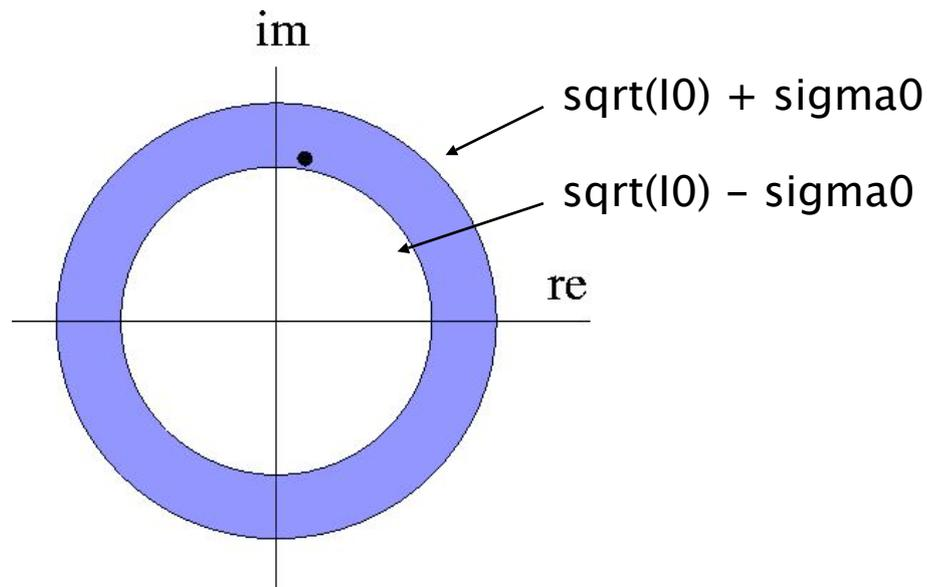
DM offset chosen to be  $\sim$  equal to speckle amplitude
