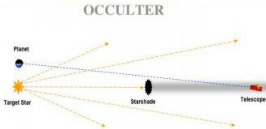
A properly placed and shaped occulter can drop a deep shadow of starlight over a telescope while allowing planet light to pass unimpeded.
