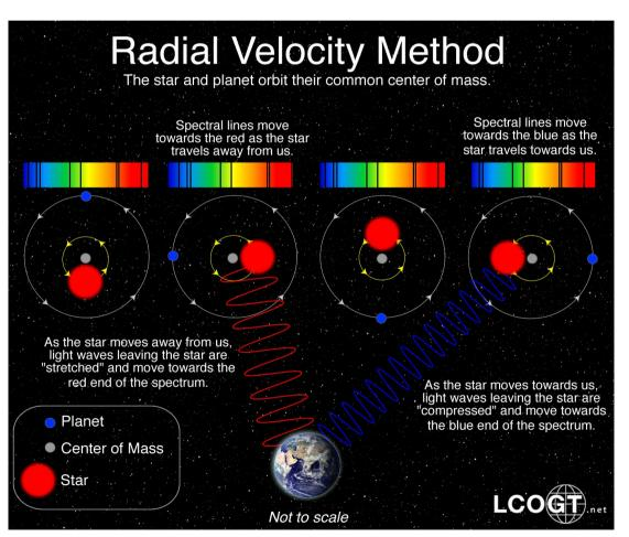
Radial velocity (RV) spectrographs can discover exoplanets and measure their masses
