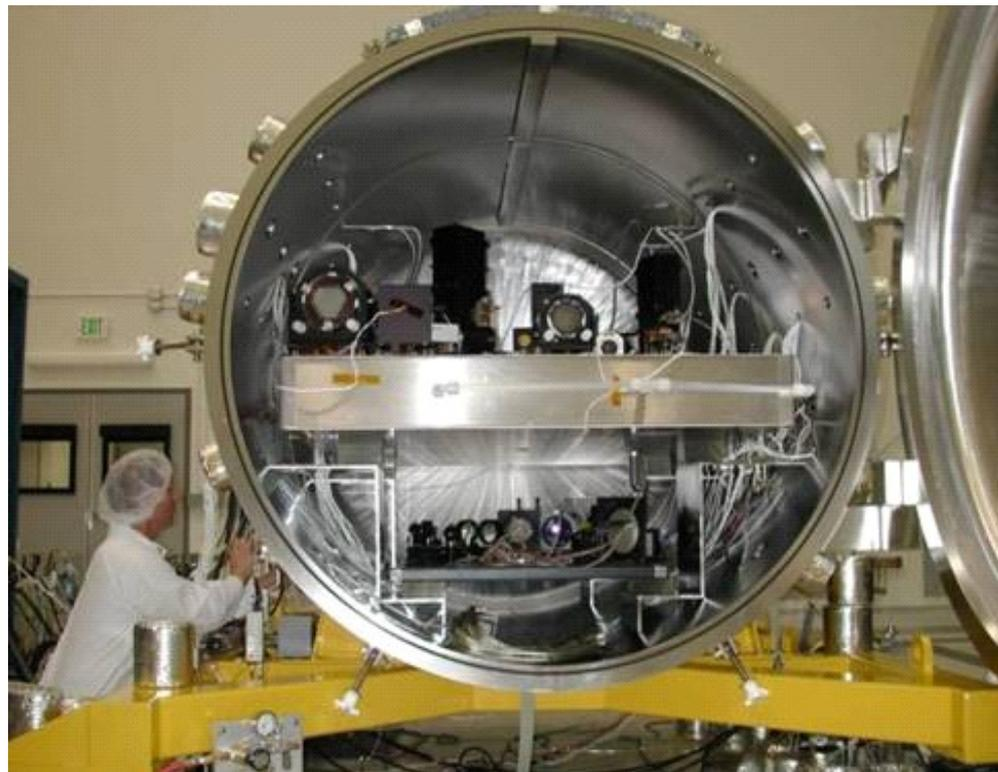
*NASA Ames testing PIAA coronagraph / WFC architectures & MEMs DMs.*
