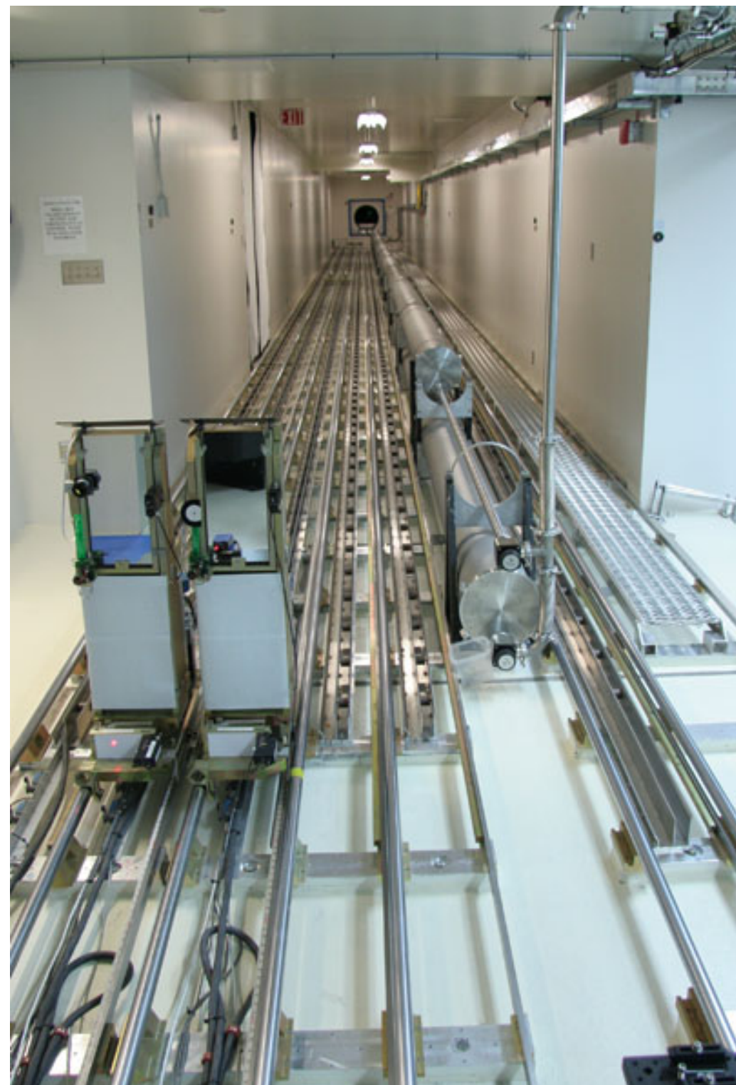
Keck interferometer coarse delay lines
