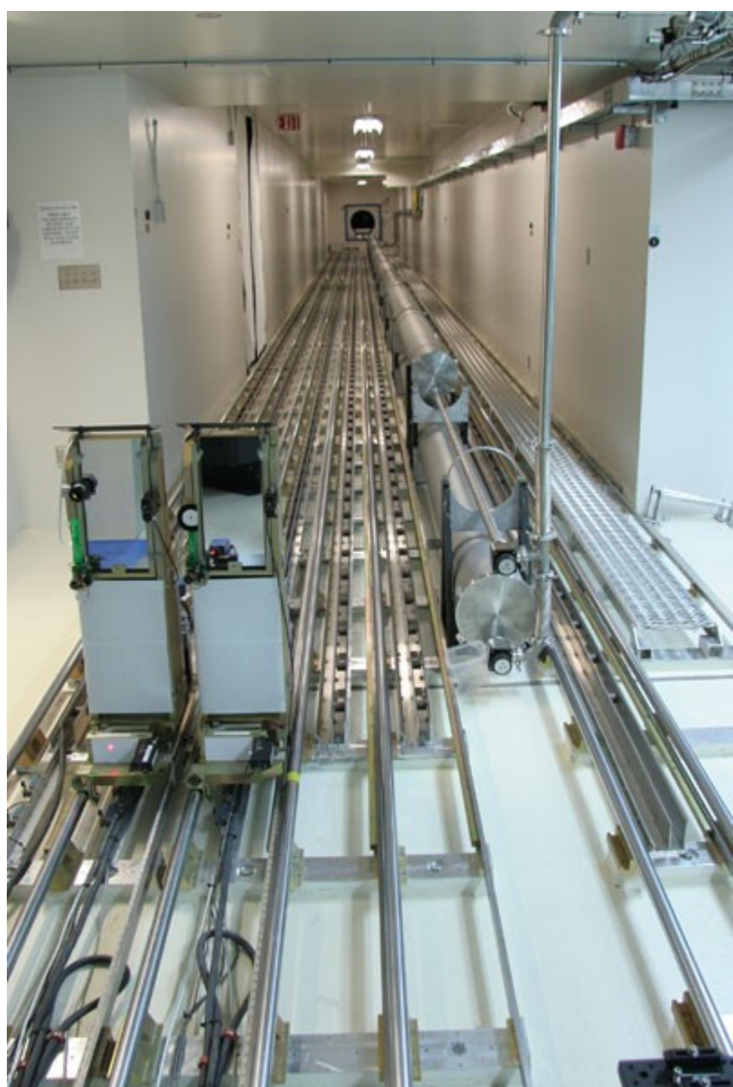
Keck interferometer coarse delay lines
