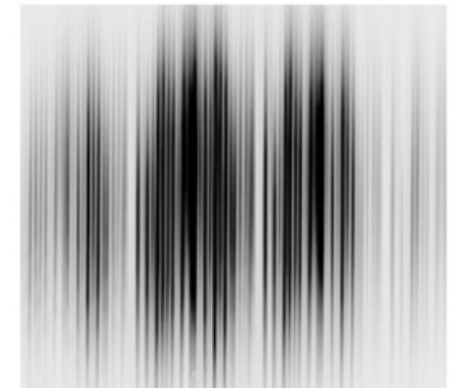
Fig.4. Left: 48 channel silicon v-groove chip from OZ optics. The fibers are arranged in non-redundantly. The fiber positions are [2,3,7,14,27,29,37,43,46]. Right: Laboratory obtained interferometric fringes using 9 fibers at a He-Ne laser.
