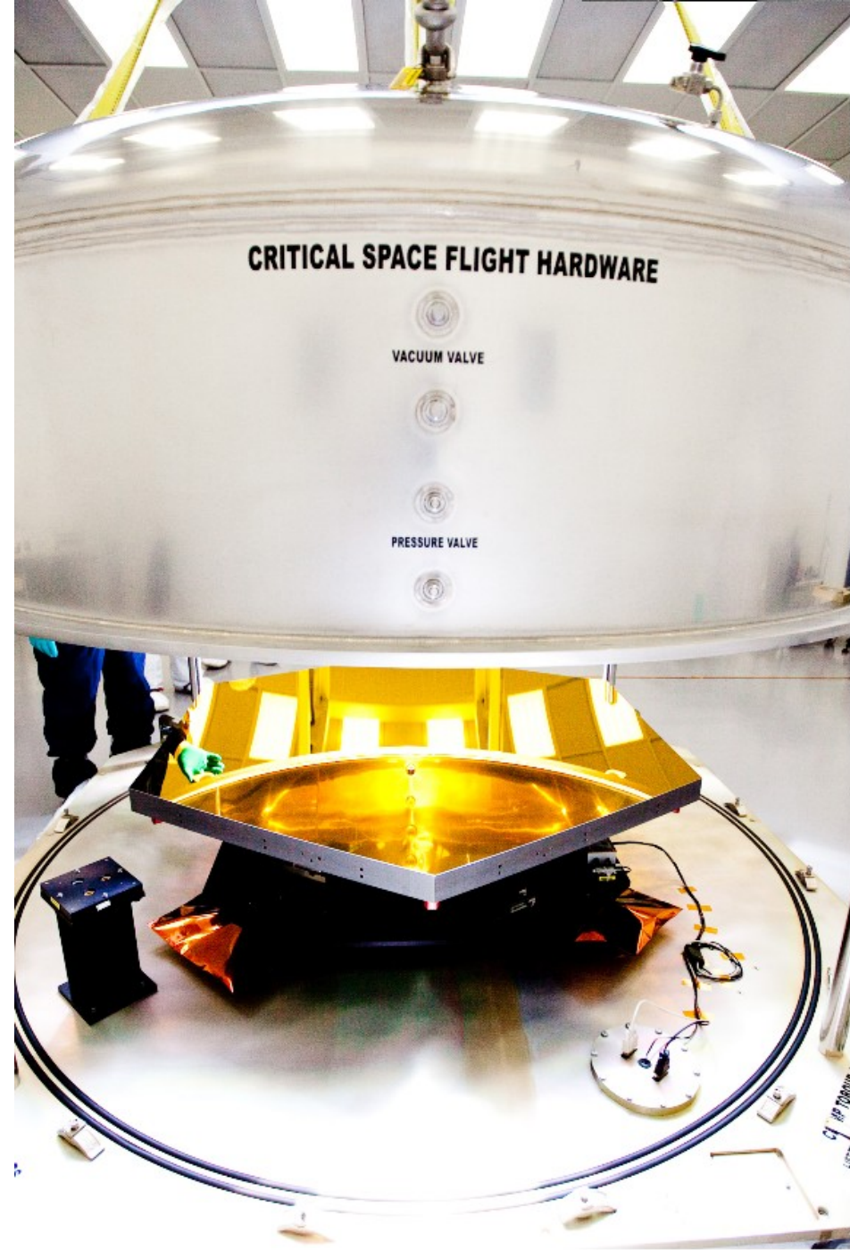
Gold-coated segment of JWST (6.5m diameter, to be launched in a few yrs)
