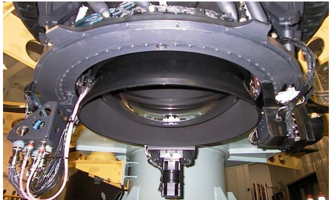
Fig. 14. Prime-focus corrector for Suprime-Cam based on a three-lens corrector design (Wynne 1965), but optimized with additional optical components for ADC.
