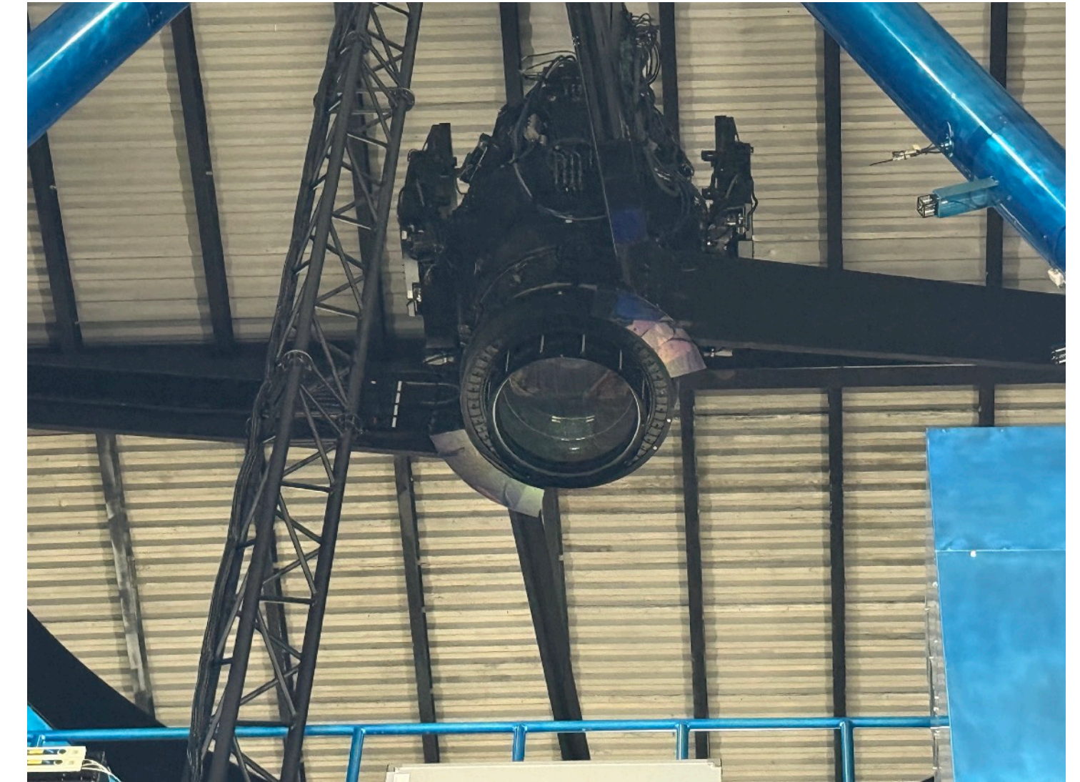
HSC mounted on the prime focus
