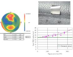
Polishing was made with a magnetorheological finishing (MRF) machine produced by QED technologies. Deviation from the designed surface is 116 nm PV. This value is confirmed to be good enough from ZEMAX simulations
