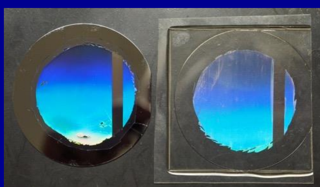
Si mold of nalux Co. Ltd. was protected by hard resin substrate.
