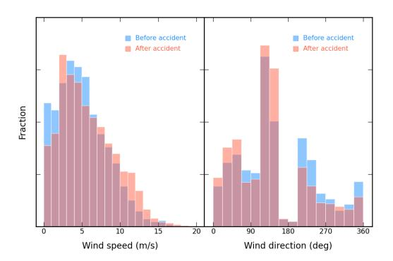
Speed and direction (AZ) distributions of the dome outside wind measured at Subaru's weather tower → There is no clear difference between these distributions before and after the windscreen accident.
