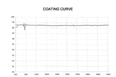
The measured reflectivity of one of the fabricated NBS mirrors. With the reflectivity of >98% at 0.45-5.0um for the five mirrors of NBS, we expect the through-put of NBS to be >90%.
