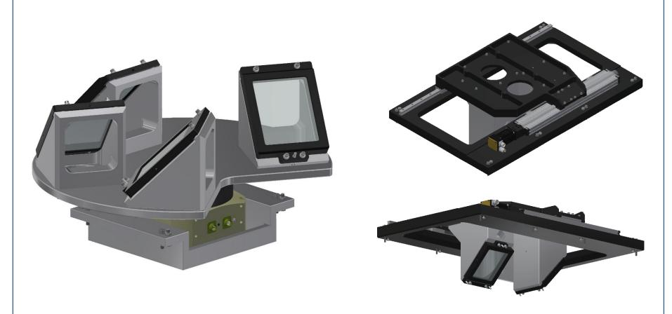
The detailed views of the switching mechanisms. (Left) The switching mechanism 1 is a rotation stage and can have 4 mirrors, dichroic-mirrors, or throughplate.
