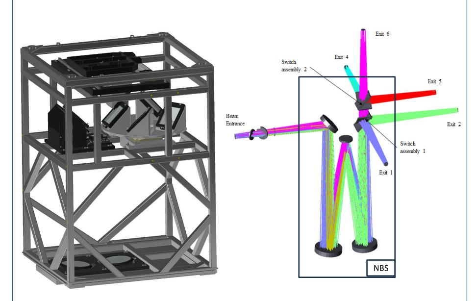
The overview of the mechanical design (left) and optical layout (right). It is composed of an Offner relay and two switching mechanisms.
