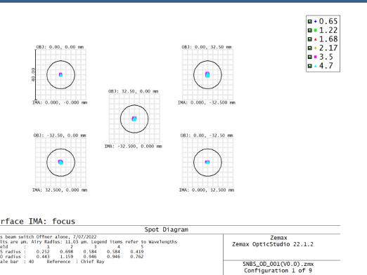
This is a spot diagram when point sources are located at the input of the NBS within the field-ofview. Their Strehl ratios are almost 100% across the full wavelength range and the field-of-view. This means the degradation of the Strehl ratio by the NBS is expected to be small.
