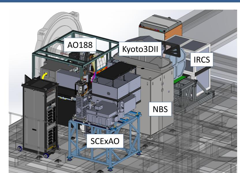
This figure shows 3D CAD model of the Nasmyth IR platform when the NBS is installed. It redirects the light from AO188 to IRCS, SCExAO, or Kyoto3DII.
