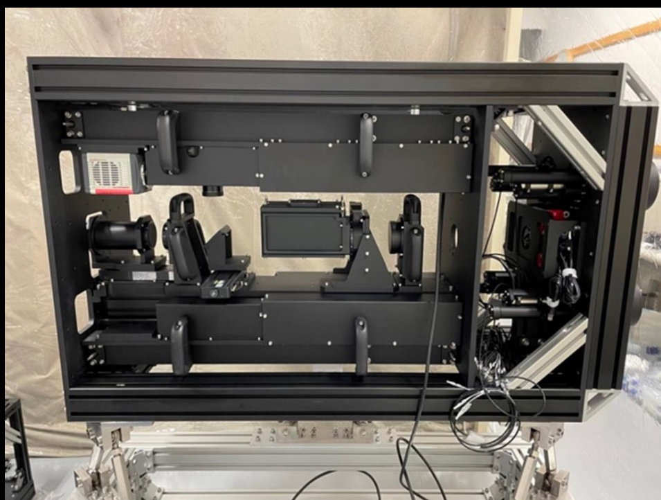
4 SH-WFS being tested at Tohoku Univ.
