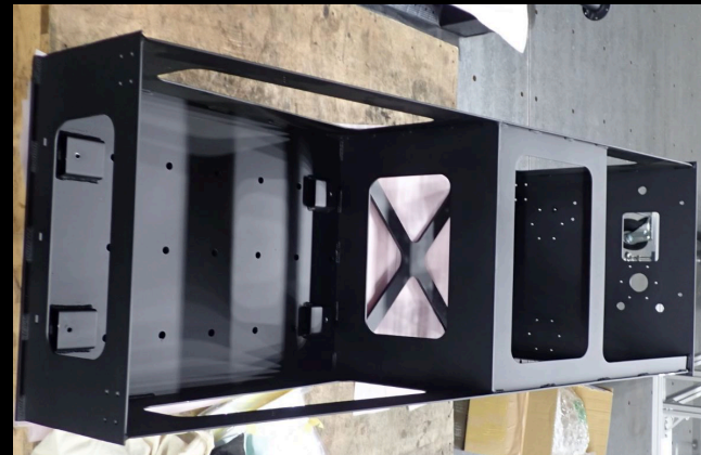
Upper truss support fabricated
