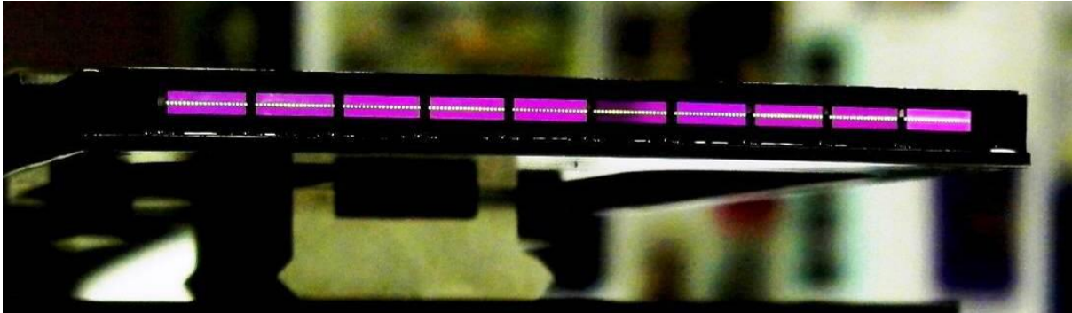
Figure 9. A slit unit during test-illumination. The line 200 of fibres can be clearly discerned, in individual blocks of 20.
